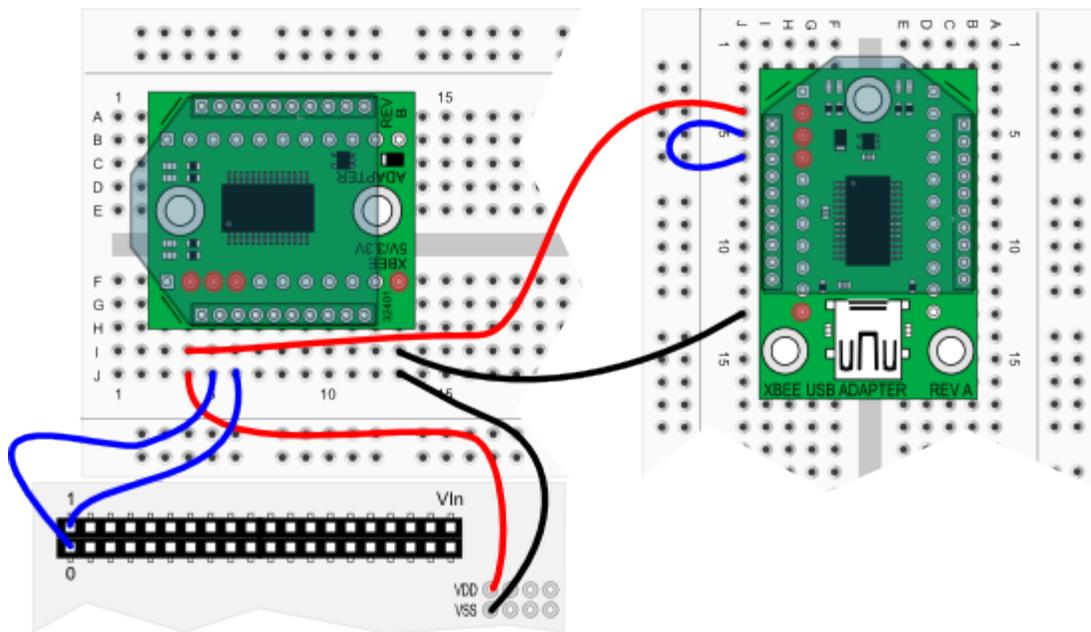
' Requires remote XBee in loopback mode (DIN connected to DOUT)
